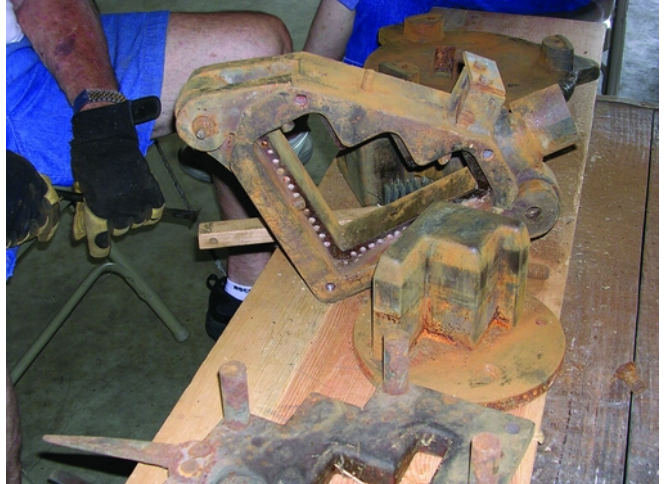
Pieces of the mold used to produce the Table Architecture candlestick.
